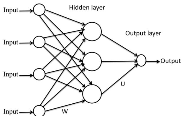
Fig. 1 A two-layer feed-forward neural network.
