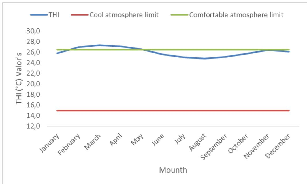
Figure 4: Inter-monthly evolution of the thermo-hygrometric index from 1971 to 2015
