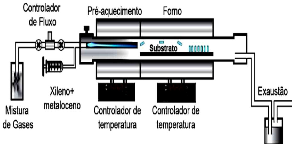
Picture 3: Schematic representation of a chemical vapor deposition reactor [(Andrews et al., 1999 and Ferreira 2003) apud SALES, 2013, p.18].
