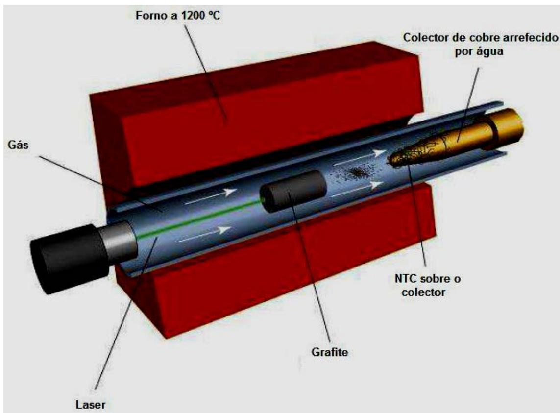
Picture 2: Representation of the procedure through the laser ablation method (Yakobson 1997 and Shibata 2011) apud SALES, 2013, p.19].
