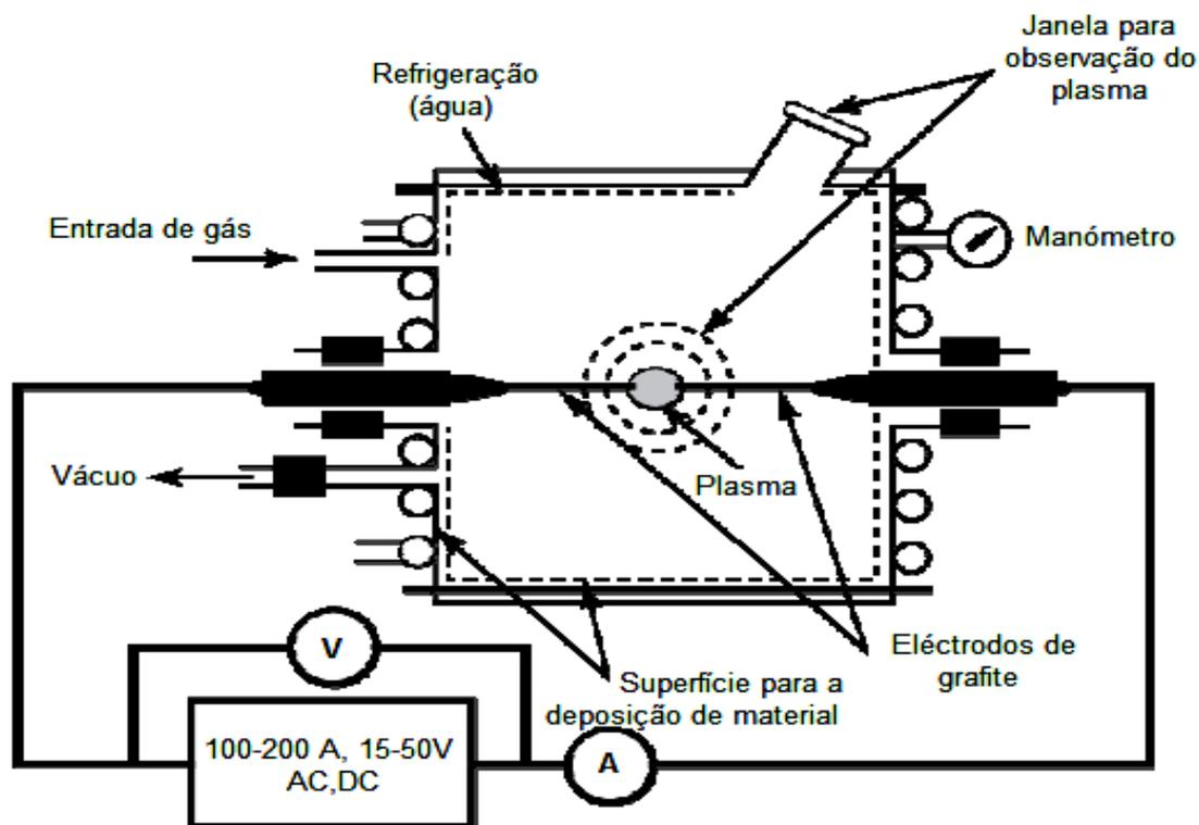
Picture 1: Schematic representation for CNT synthesis by current arc discharge [Journet and Bernier 1998 and Ferreira 2003] apud SALES, 2013, p.17].
