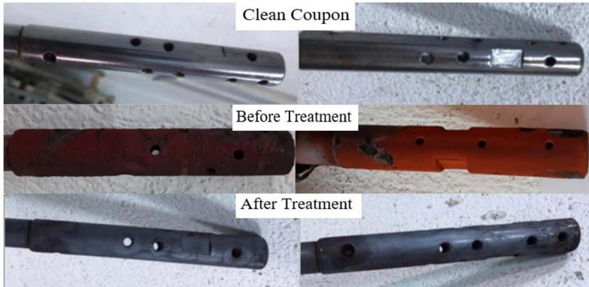
**Figure 4.** Preheater Output Coupons
