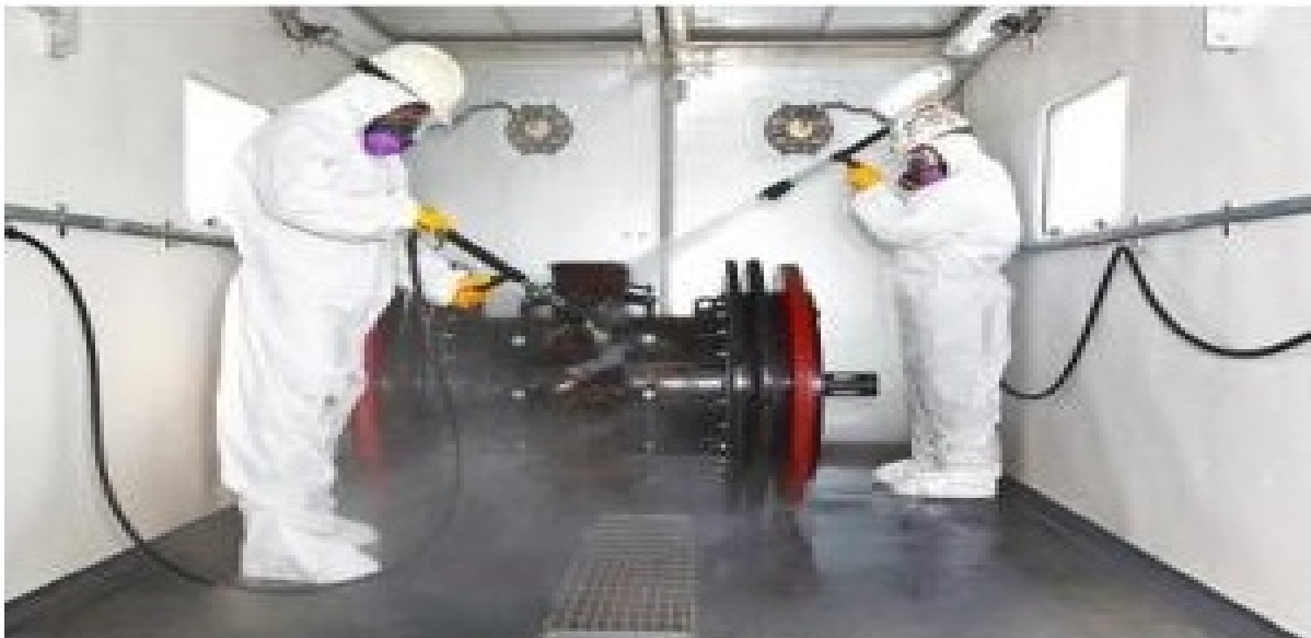
Figure (12) shows the appropriate outfit for oil workers when cleaning the pipes and equipment(3).
