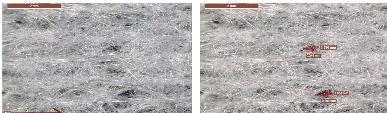
Figure 3. Pattern Image of Spunlace Nonwoven Fabric and Gaps in Fibers (Leica S9i Microscope 10x Magnification)
