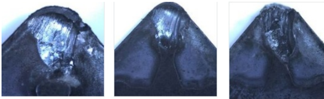
Fig – Wear of Cutting Edge 300m/min, 400m/min and 500m/min (Costa, 2016)
