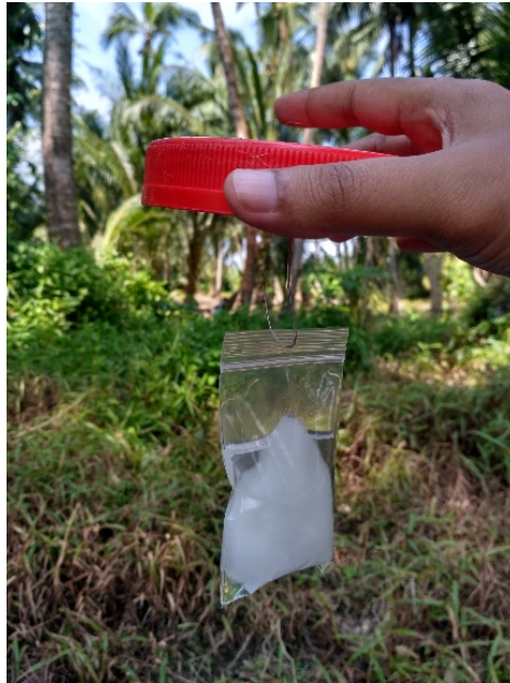
Figure 7. Ethyl acetate soaked in cotton wool and place in zipped plastic bag as dispenser
