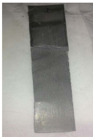
Figure 3b. Shape of aluminum after electrocoagulation
