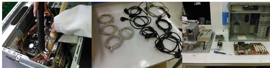
Fig. 5 TR7.1: Internal cleaning of hardware (left), classification of cables (center) and components (right)
