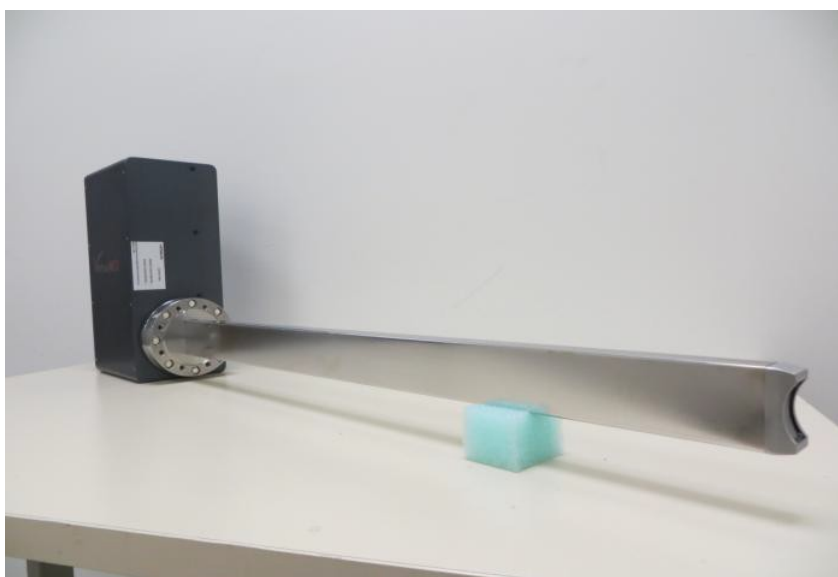
Fig. 8. The Vortex ® ME-3, three 50 mm 2 SDDs, focal design: focal point at 30 mm.
