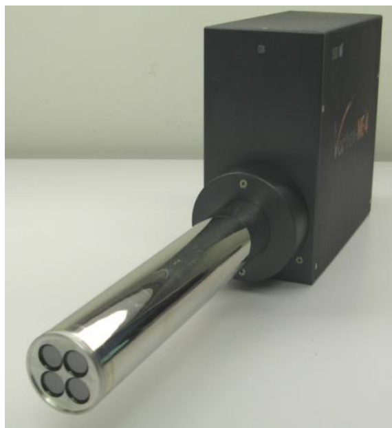
Fig. 7. The Vortex ® ME-4, containing four 50 mm 2 SDDs, for synchrotron high count rate applications
